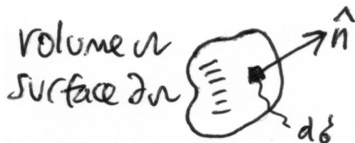
Figure 9: Construction for use in studying the continuity equation. A volume \Omega is bounded by the surface \partial\Omega . At a given point on the surface, \hat{\mathbf{n}} denotes an outward-pointing unit vector that is normal to the surface, while d\sigma denotes an infinitesimal element of area.
